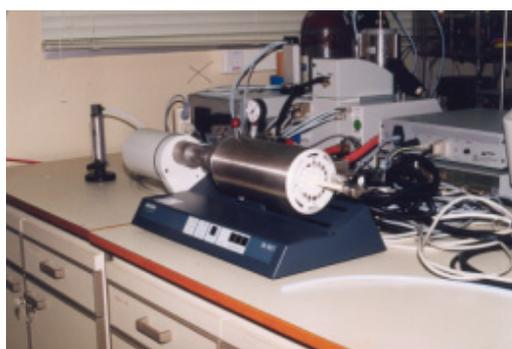
**Figure 2:** Therm dilatometry equipment, NETZSCH model DIL 402 C.
