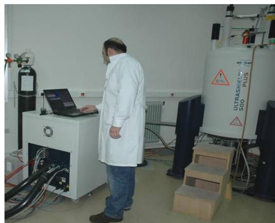
**Figure 6:** The cryo-unit that is connected to the cryo-probe at the AV500 system.
