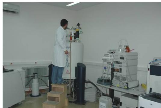
**Figure 5:** General view of the Brücker AV-500 spectrometer (resonance frequency of  $^1\text{H}$  500 MHz) and the LC-SPE system.
