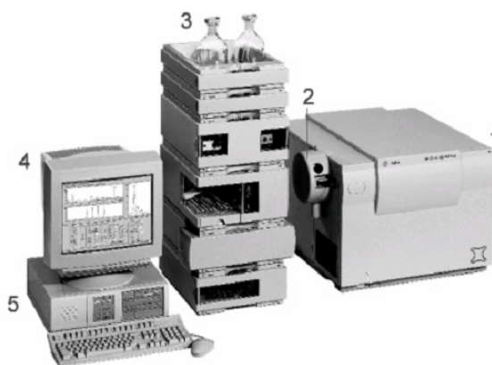
Figure 1: General view of the low resolution Agilent 1100 Series LC/MSD Trap System. Ion trap mass spectrometer (1) with its interface (2), the Agilent 1100 HPLC system (3), monitor (4) and computer (5) are shown, only.
