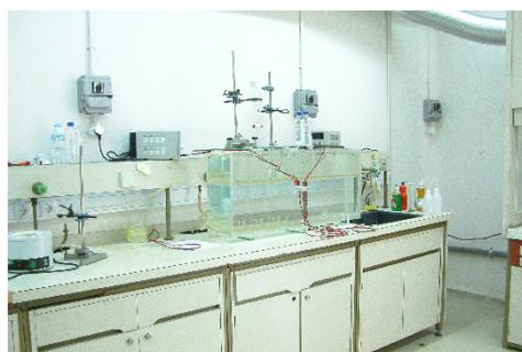
**Figure 3.** Electrolysis equipment for tritium enrichment.
