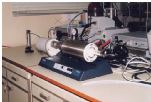
**Figure 2:** Thermodilatometry equipment, NETZSCH model DIL 402 C.
