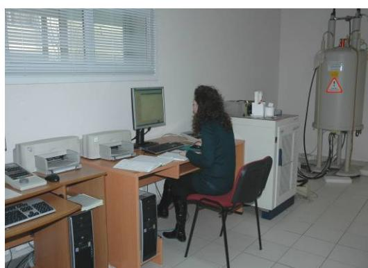
**Figure 4:** General view of the Brücker AV-400 spectrometer (resonance frequency of  $^1\text{H}$  400 MHz).
