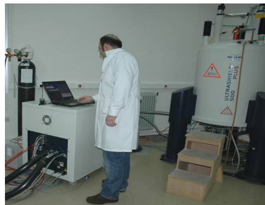
Figure 6: The cryo-unit that is connected to the cryoprobe at the AV500 system.
