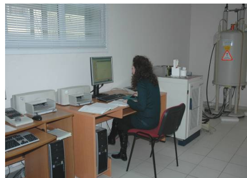
Figure 4: General view of the Brücker AV-400 spectrometer (resonance frequency of ^1\text{H} 400 MHz).
