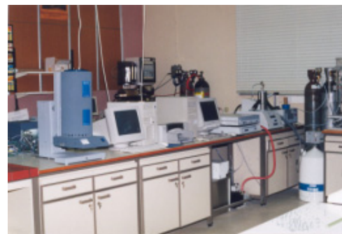
Figure 1: The STA 449C JUPITER equipment that combines TG/DTG, DTA and DSC techniques (on the right) and the SETARAM C80 calorimeter (on the left).
