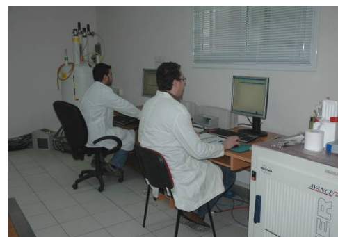
Figure 3: General view of the Brücker AV-250 spectrometer (resonance frequency of ^1\text{H} 250 MHz).
