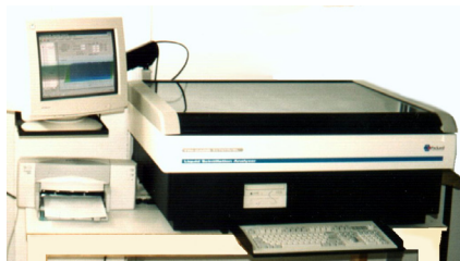
Figure 1: General view of the temporary installations of Tricarb 3170 TR/SL liquid scintillation counter.
