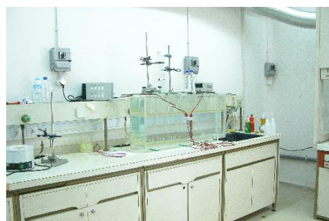
**Figure 3.** Electrolysis equipment for tritium enrichment.
