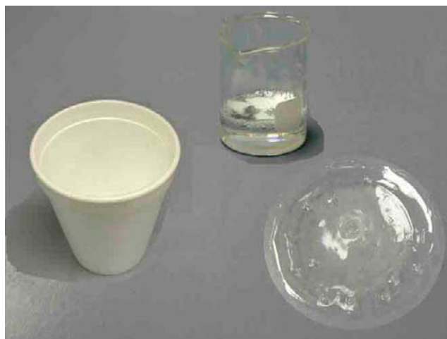
FIGURE 7. Polystyrene cast peeled off of a watch glass (right) after evaporating the toluene or acetone solution (centre) of a Styrofoam cup (left).
