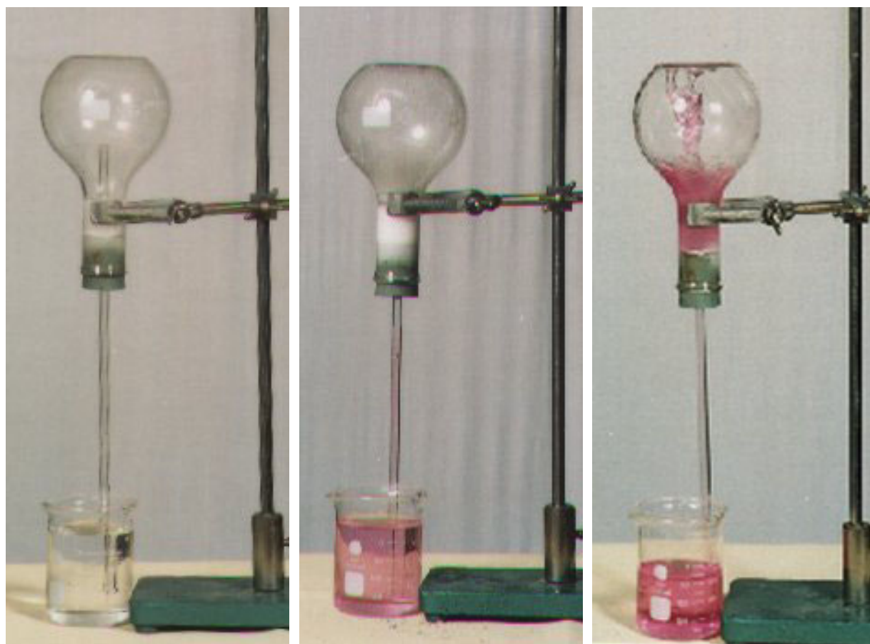
FIGURE 1. Experimental set-up, and three instances of the ammonia-fountain experiment.
